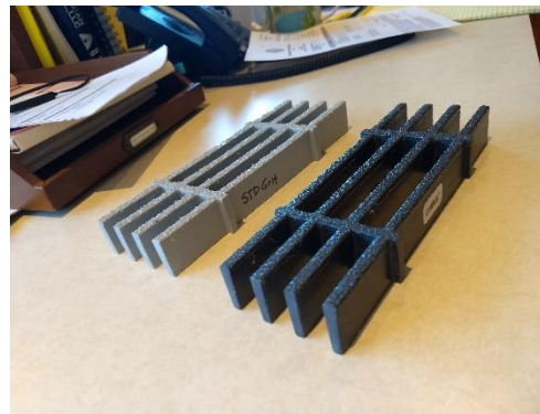
Fiberglass Grated and Gritted Float Surface
